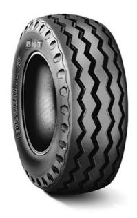
**Description** INDUSTRIAL RIB F3 is an agro-industrial rib-pattern tire designed for field and road transport as well as for soil
