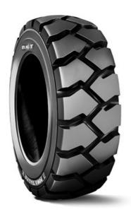
POWER TRAX HD is a premium bias-ply tire that is specially designed for forklift equipment in industrial applications. The deep tread, the extra thick sidewall and the tough casing provide exceptional durability minimizing the risk of punctures and accidental damages. The tire features excellent cut, chip and tear resistance suitable for rough and hard concrete surface.
