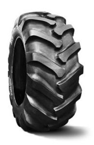
**Description** TR 678 has been specially designed for forestry applications. Its robust lug design provides excellent
